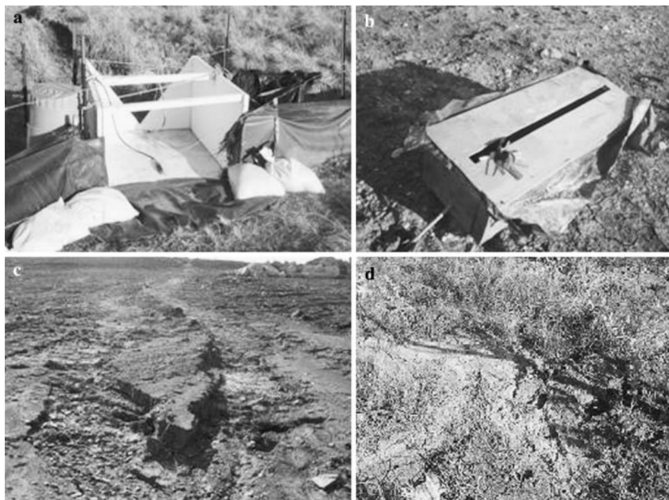
Fig. 3 a A V-notch weir installed at the Site 2 reference site. Plastic sheeting funnels runoff through the weir. The floor of the weir, several cm below the notch, acts as a partial sediment trap capturing bed load and some suspended load sediment. b Bed load trap. A plastic-lined, plywood box with a slotted metal cover is buried in the bed of a channel. Sediment is trapped when it falls through the slot
